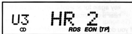
Display during hands-free operation, when a Traffic Announcement is broadcast via RDS-EON
